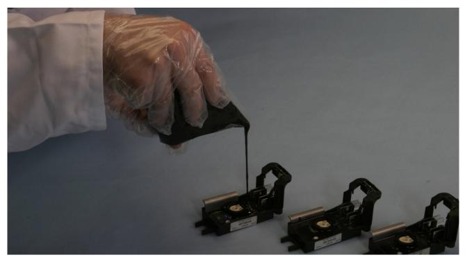
A leading Spainish company specialising in innovative smart metering solutions for water and gas meters is using EL199HP for potting electronic RFID transmitting data devices for mechanical water metering devices.
